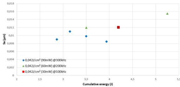
**Fig.6** Analysis of LIPSS surface roughness as a function of cumulative energies
