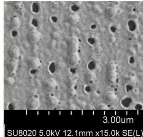
**Fig.8** SEM analysis for LIPSS with 0,042J/cm², 80mm/s 300kHz
