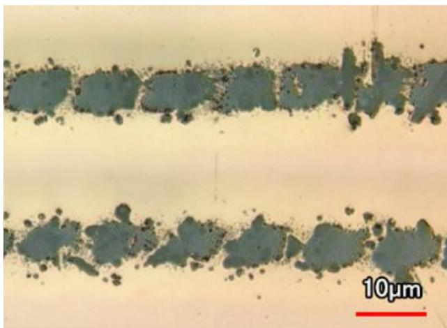
Fig. 3 Ablation of the thin gold layer obtained with a fluence of 0.09 J / cm<sup>2</sup>
