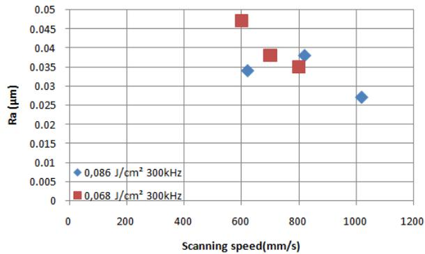
**Fig. 9** Linear Roughness Ra vs scanning speed for 6 different parameters showing periodic ablation
