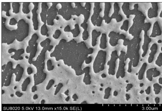
**Fig. 11** SEM analysis for Periodic ablation for LIPSS with 0,086J/cm².
