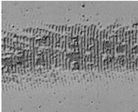
**Fig. 10** Periodic ablation for LIPSS with 0,086J/cm², 300kHz, 820mm/s.
