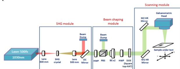
Fig. 1 Laser experiment for LIPSS structuring
