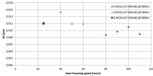
**Fig.5** Analysis of LIPSS surface roughness as a function of scanning speed, for 3 different laser repetition rates
