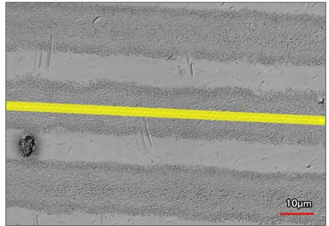
**Fig.7** Analysis for LIPSS with 0,042J/cm² with a laser scanning speed of 80mm/s, 300kHz
