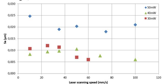
Fig.4 Analysis of LIPSS surface roughness as a function of the scanning speed, for 3 different laser powers @100kHz
